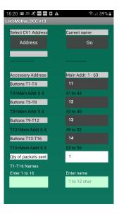
These may be changed to suit your accessory decoder for turnouts/points etc. Example here shows main address of 11 to 14 which will operate decoder addresses 41 through 56
